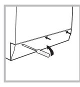
1. using a screwdriver, remove the cover panel on the lower front part of the washer-dryer (see figure);
